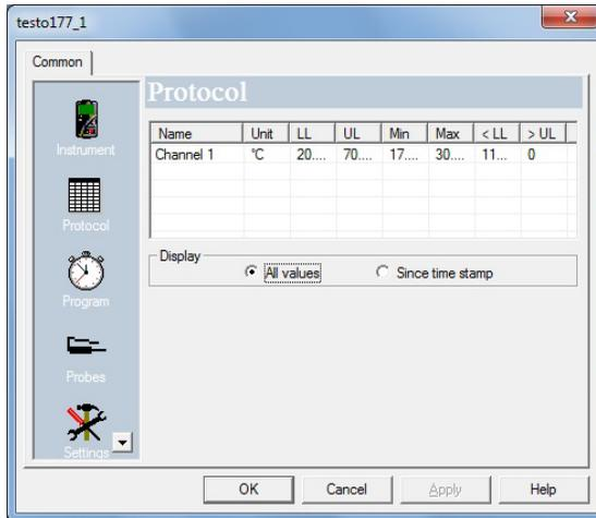
The window **Protocol** only appears if a measuring program has been performed and has been saved in the instrument.
